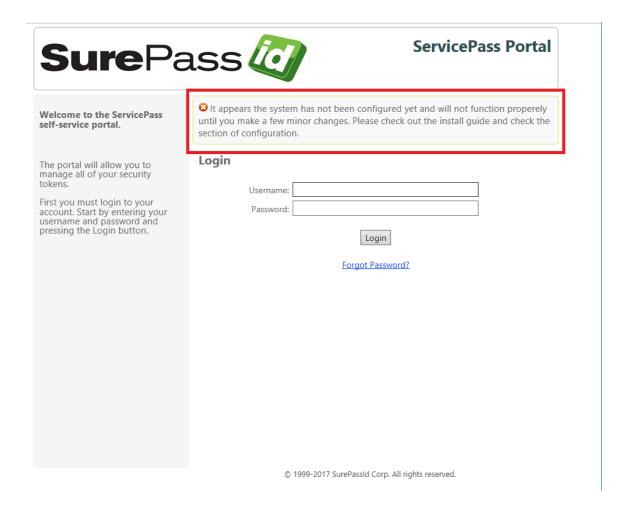
This screen informs you that the system is installed and ready and needs to be customized before it can be used. Once you customize the system, this message will no longer appear. The next section will provide you with the information you need to customize the system to use your instance of SurePassID Authentication Server and specify default functionality for your user base.
